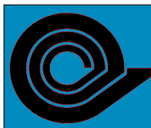
PCB Winding Patterns, Circular Shape (Top View)
