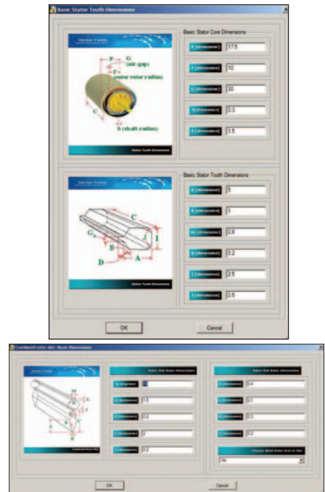
Figure 1. Dialog window requesting information for the stator (top) and the rotor of the induction motor.
